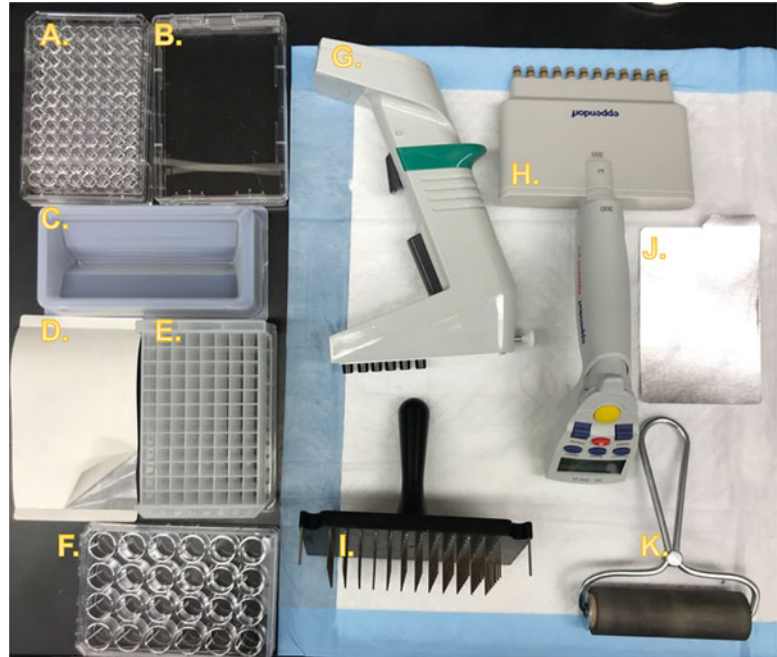
Fig. 2 Equipment and consumables for Replica Set experiments. Equipment necessary for RSM experiments is commonly available in laboratories that work with C. elegans , especially those which regularly utilize feeding-based RNAi. (a) 96-Well culture plate for storage of frozen libraries of bacterial RNAi clones as glycerol stocks. (b) Rectangular single-well plate for LB amp + tet agar slabs for creating intermediate-term working cultures of RNAi libraries on solid media. (c) Reagent reservoir for bulk reagent pipetting tasks with multichannel pipettes, such as adding fresh LB to a new 96-well plate. (d) Gas-permeable adhesive membrane for sealing deep-well plates during incubation while allowing gas exchange. Note that in the image a corner of the backing has been peeled back to reveal the membrane. (e) 2 mL deep-well culture plate for seeding replica plates. (f) 24-Well culture plate for use as replica plates. In a typical experiment, wells would be filled with solid RNAi growth media before seeding with bacteria and then C. elegans . (g) Electronic 1250 \mu\text{L} six-channel repeat pipette with adjustable tip spacing (sometimes referred to as an “equalizer” pipette). (h) Electronic 300 \mu\text{L} 12-channel repeat pipette (fixed spacing). (i) Pin plate replicator for 96-well plates with stainless-steel pins. Allows easy transfer of bacteria from glycerol stocks to liquid culture, or from liquid culture to solid media, while also being easy to sterilize. (j) Adhesive foil cover for frozen RNAi library glycerol stock plates. (k) Rubber roller for securing adhesive foil plate covers
