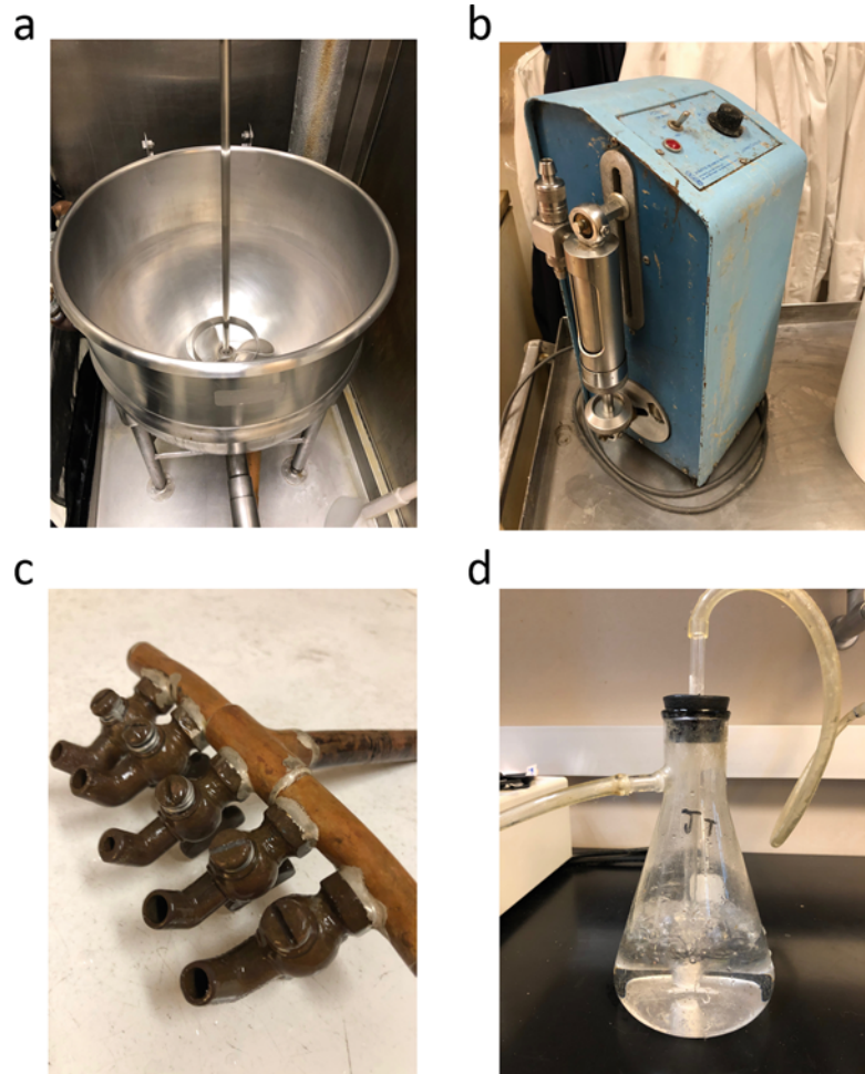
Fig. 1 Equipment. (a) Steam-jacketed kettle. (b) Pump. (c) 5-headed nozzle. (d) Bubbler
